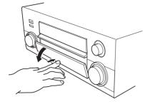
**12 ACOUSTIC CAL.** (page 44) Press to switch Acoustic Calibration EQ on or off.
